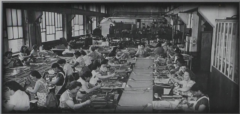
African Americans relocating to Erie from other parts of the U.S. sought employment in the city’s thriving industrial sector. Women working in General Electric’s Building #6, wrapping coils with insulating material, 1950s or 60s. Courtesy of Sylvia Thurston
